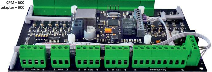
If you use a wire other than the supplied wire, do not exceed the maximum wire length of 50 cm (I2C bus). All 4 COM.i2c terminals on the CPM are equipped with an optocoupler with galvanic isolation from the BCC, so there is no risk of potential difference damage if the BCC unit is powered, for example, by a switching power supply from a source other than the CPM.
