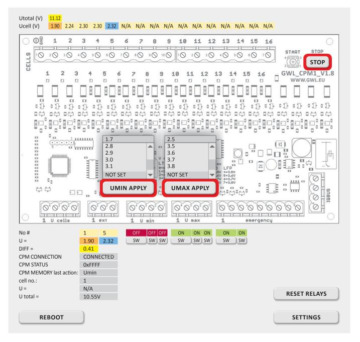
Below the figure there is the maximum cell voltage and the order of this cell in the battery, the minimum voltage and the order of the cell in the battery, the difference between the maximum and minimum voltage, communication status with the CPM and any error code.
