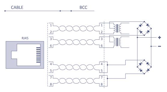
Therefore, the DC supply voltage up to 65V can be applied to the pairs of UTP cable number 1 + 2 (orange and white-orange), 3 + 6 (green and white-green), 4 + 5 (blue and white-blue) and 7 + 8 (brown and white-brown) regardless of polarity.
