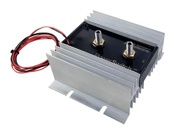
The PowerSwitch is a bidirectional solid state relay with very low power consumption when turned on. This will ensure that it can operate for a very long time, even if the battery is almost empty. A second benefit is that it can switch bidirectional currents. This means that it can be used with devices which both can charge and discharge, like a combined charger/inverter.
