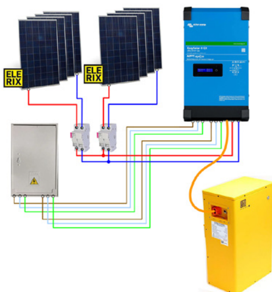
Single-phase hybrid PV plant
