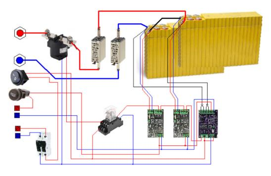
In more advanced systems, an independent 24V DC backup power supply for the control circuits is available. This can be used to power the EasyT module, the power contactor, and its auxiliary relay. The robust and durable BMS Easy system without software can have, for example, a basic (backup, emergency) function alongside of an advanced digital superstructure.
