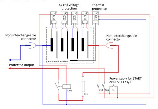
If a cell goes out of the allowed voltage range or the temperature of the cell block exceeds the allowed temperature, the relay on the corresponding Easy module switches to the NC position, and contactor KM1 loses voltage on the coil and disconnects the power.
