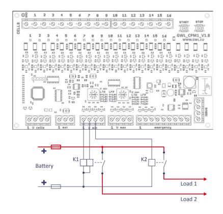
Connect high dispensable load via a standard relay, indispensable via a bi-stable relay. The high load will be disconnected first, and if the cell voltage is stable within 20 s, the important load will no longer be disconnected.
