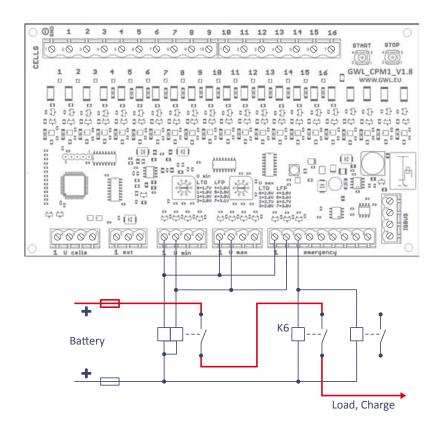
For each protection (Umin Umax Uemergency), it is advisable to use a separate relay for maximum battery protection. The combination of two or three pulse outputs per bi-stable relay reduces the quality of protection (possibility of contact bonding, coil or output failure, etc.). The combination of pulses can be used in justified cases; the electrical module structure makes it possible.
