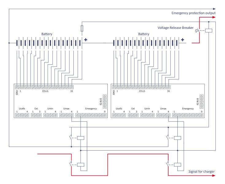
Batteries consisting of more than 16 cells must use additive connection of the CPM. Auxiliary relays must be used to control the disconnecting elements and status signalization.
