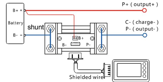
**Attention:** Please connect as shown strictly. The shunt must be connected to the negative circuit, it is forbidden to connect to the positive circuit. If you want to extend the shielded wire, you must use 4 lines of same specification.
