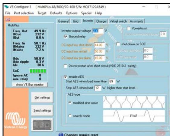
After making all of these changes, press the “Send settings” button. The VE device will ask to restart. Restart to complete the set up. It is best to perform a cold boot
