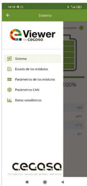
**6. Module status:** This window shows the number of modules in the system (in this case 3) and if any of them have a Warning or Alarm. In which case the cause of the Warning or Alarm is shown.
