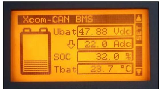
This shows the battery’s voltage, current, SOC and temperature. These values are the ones that the TCC-CAN sends the inverter via CAN communications. If the above variables are showing a value (similar to the above image) then this means it is communicating correctly. If there is no communication, then the **Xcom-CAN BMS** screen will not appear or appear without any values (see image below).
