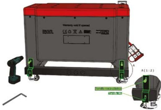
d) When mounting TWO modules, the front of the modules have to be fastened together using the fastening plates (long flat) and screws that are supplied with each of the modules. An ALLEN key is required.
