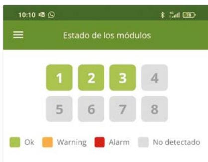
**7. Module parameters:** This window shows different information about each of the batteries that form the system.
