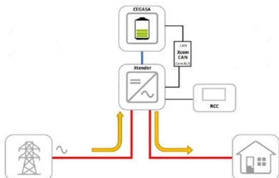
In this example, the mains supply has been connected to the Xtender inverter as AC In input and an AC output charge. On the DC side, a Cegasa battery system has been connected to the TCC-CAN.
