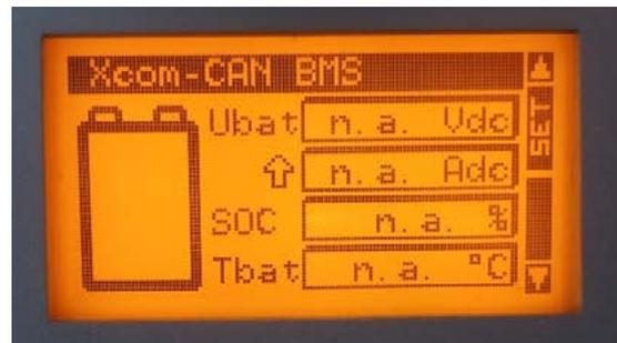
Once correct communication is established, it is possible to check the values of the other variables sent by the TCC-CAN. To do this, follow these steps on the Xcom-CAN BMS screen:
