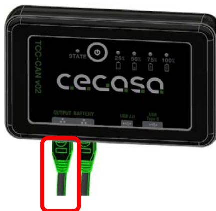
**Note;** If there is no communication with the inverter at this point, then disconnect the cable that goes to the "battery" position on the TCC, wait 5 seconds and reconnect it. This basically resets the communications.
