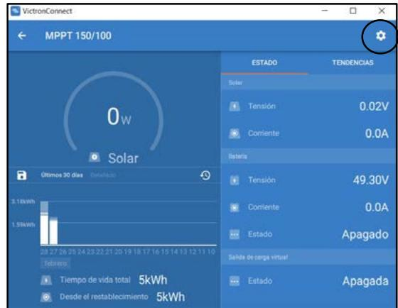
Select Battery / Battery Pre-set / User Defined and then modify the following parameters (as shown in the image).
