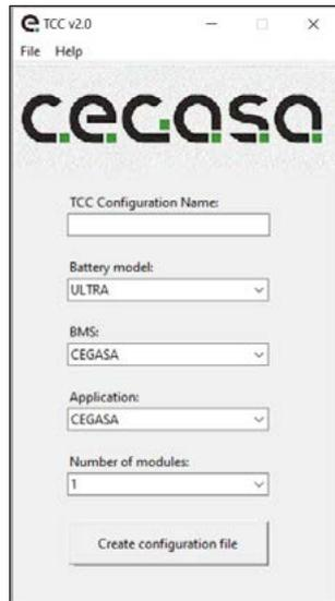
2.3. In the “TCC Configuration Name” field, write the name of the folder that is going to contain the configuration file (E.g., “EXAMPLE”). After which, choose the path where it is going to be stored.
