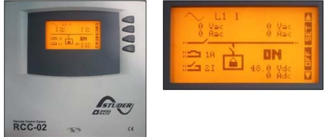
From the main screen, pressing the “down” button selects the screen to be displayed on the console. To view the battery’s most important variables, select the **Xcom-CAN BMS** screen, as shown in the image below.
