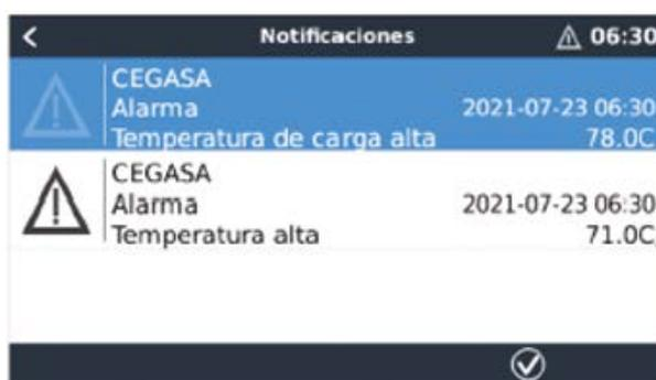
The **Warning** symbol will flash while the alarm is active and be semi-transparent and not flashing if the alarm has been reset. Even if the system is active again, the notification remains on the screen so that the warning (not the system) can be reset manually.
