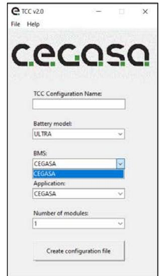
1.6. The “Application” field has a drop-down menu. Use this drop-down to select the corresponding inverter model or application. In this case **Victron**.
