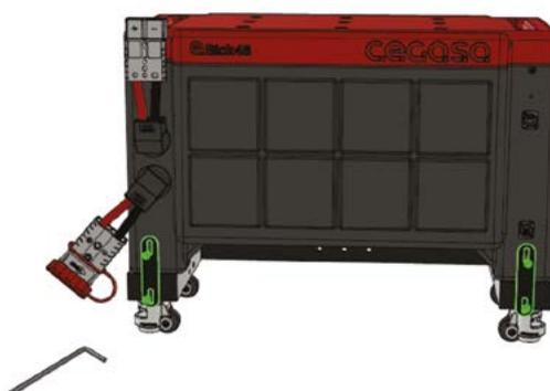
c) At the back, fasten the module to the base frame using the two plates (bent) and screws (2 metric threads - bottom and 2 plastic threads - top) supplied with the base frame assembly. An ALLEN key and screwdriver are required.
