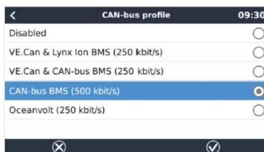
In the main menu, go to **Device Lists / Settings / Services / BMS-Can port / Select Profile CAN-bus BMS (500 kbit/s)**
