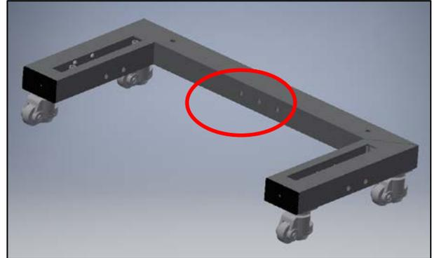
g) In the event that several columns have to be joined together, this is also possible by using a nut-bolt connection through the 2 x Ø10mm holes that are on the sides of the base frame, once the equipment is in position.
