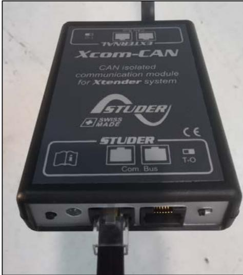
The part labelled **EXTERNAL** is connected to the TCCv2.0-CAN by using another Ethernet cable. Note that the position of the T-O switch must be the same as shown in the image.
